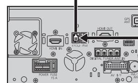
ETC2.0車載器接続端子へ
